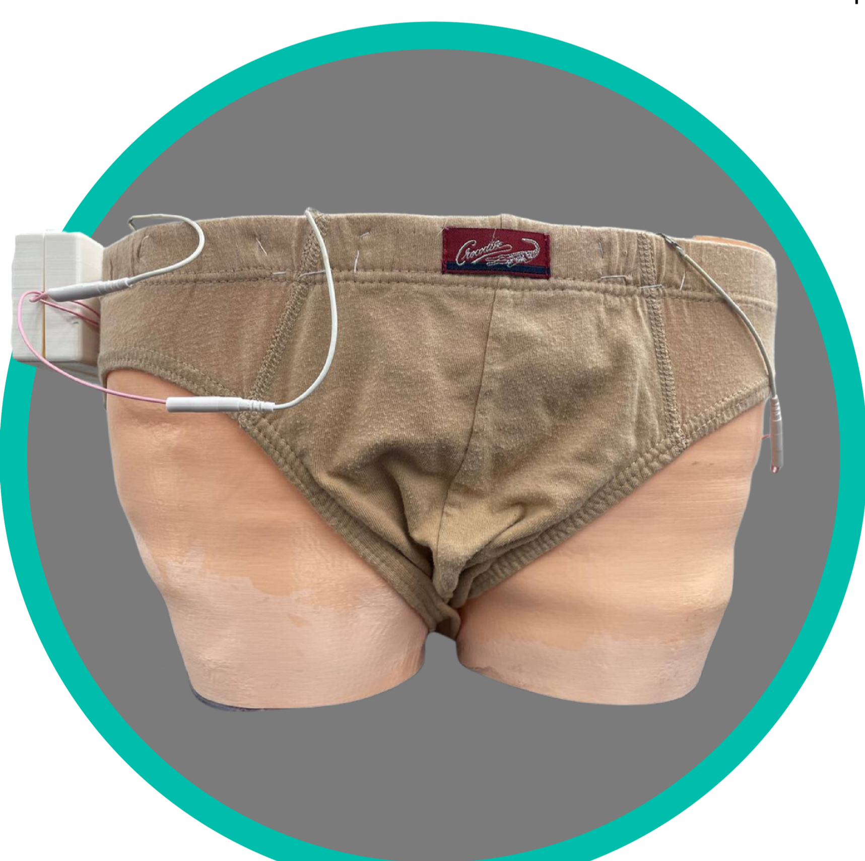
Multi-frequency impedance analysis using phantom bladder and urine
